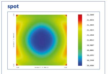
• spot radius in μm at 86% level for a Gaussian laser beam (M<sup>2</sup>=1) with 12 mm diameter at 1/e<sup>2</sup>, clipped at 1/e<sup>2</sup>
